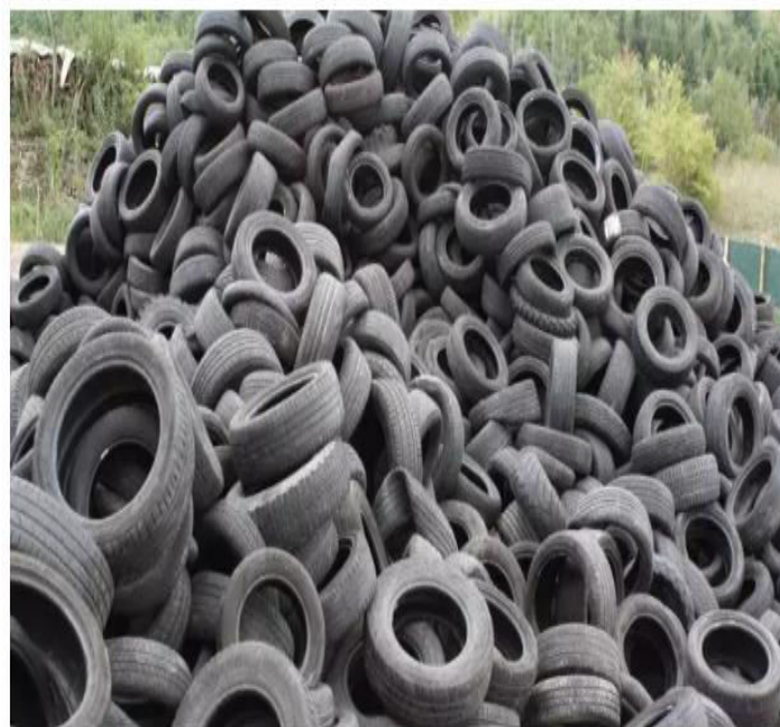
The waste tyres are recycled as reclaimed rubber, crumb rubber, crumb rubber modified bitumen (CRMB), recovered carbon black, and pyrolysis oil/char.
